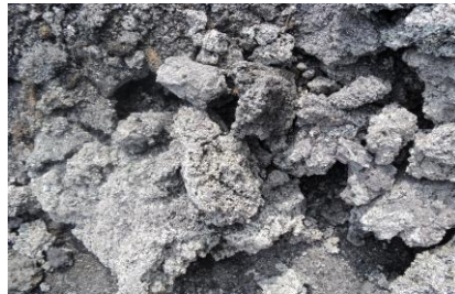
Figure 1 Palm oil clinker produced after burning the palm oil fibre and oil palm shell with high temperature.
