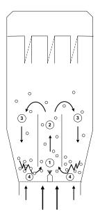
Figure 2. Schematic drawing of the fluid bed with Wurster technique
