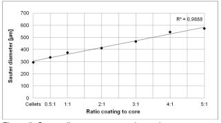
Figure 5. Sauter diameter versus ratio coating to core
