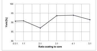
Figure 3. Yield of coated pellet lots versus ratio coating to core
