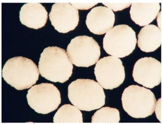
Figure 4. Stereo microphotograph of sodium benzoate loaded pellets, ratio coating to core 3:1
