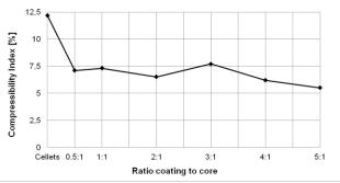
Figure 9. Compressibility index versus ratio coating to core
