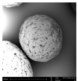
Figure 10. SEM of coated pellet lot, ratio coating to core 0.5:1, sphericity 0.949
