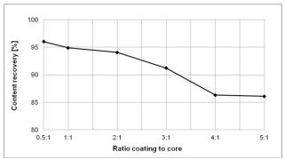
Figure 12. Sodium benzoate recovery rate versus ratio coating to core
