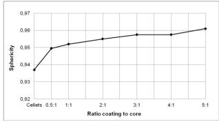
Figure 7. Sphericity versus ratio coating to core
