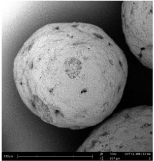
Figure 11. SEM of coated pellet lot, ratio coating to core 4:1, sphericity 0.958
