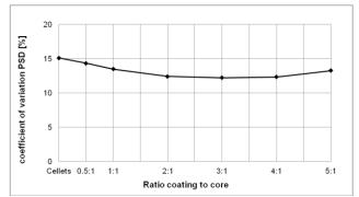
Figure 6. Coefficient of variation of Sauter diameter versus ratio coating to core
