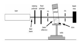
Figure.1 : The optical system setup of Mie scattering[12]
