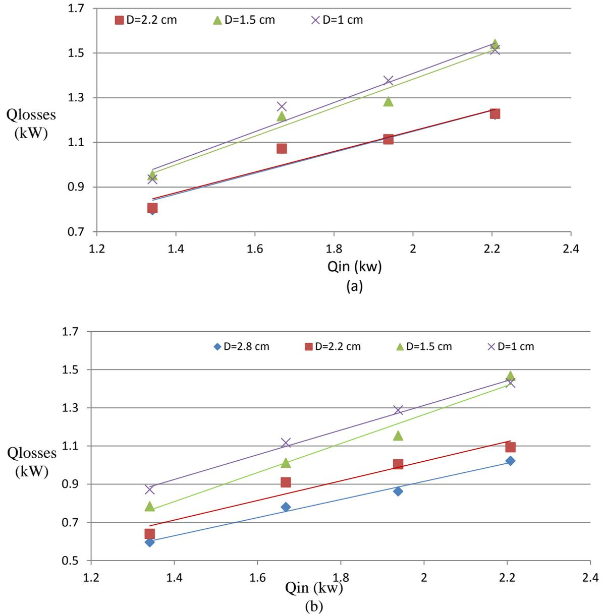
Figure 5. Curves represent the relation between heat losses with heat input to the fire tube heat exchanger for different tube positions (a) position 1, (b) Position 4.
