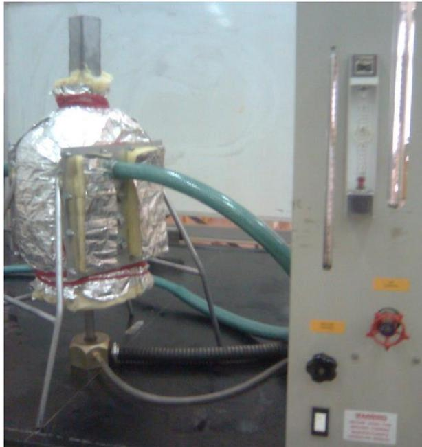
Figure. 4. Actual chimney type Fire Tube Heat Exchanger equipped with Flame Propagation and Stability Unit to control the combustion process.
