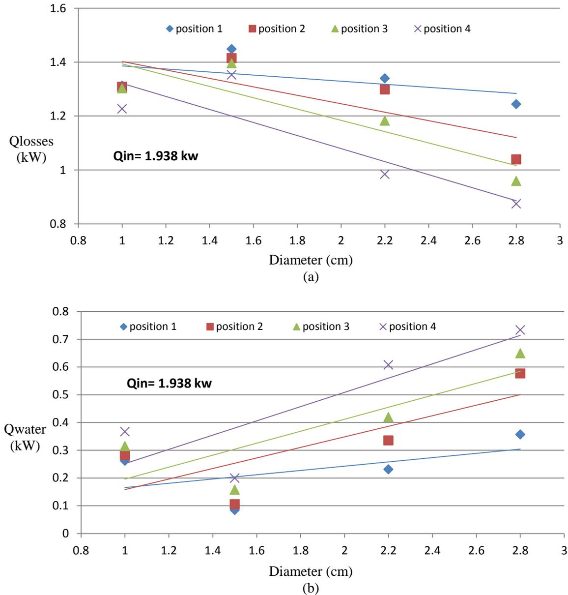
Figure 7. Curves represent the effect of tube diameter on (a) heat losses, (b) water heat gain.
