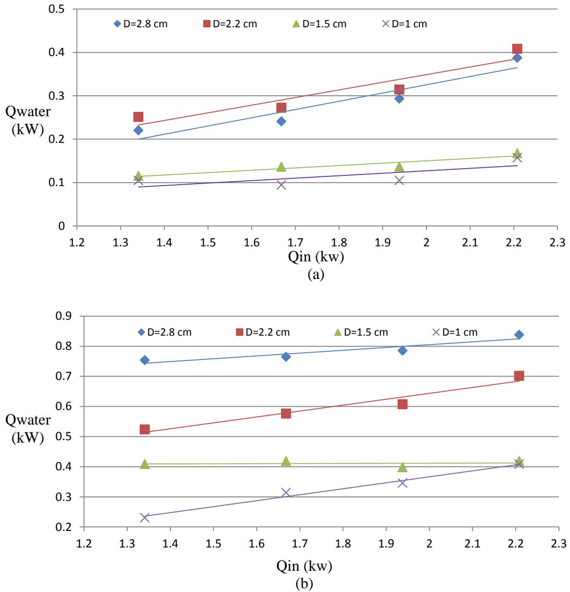
Figure 6. Curves represent the relation between heat inputs with heat transferred to water in the fire tube heat exchanger for different tube positions (a) position 1, (b) Position 4.
