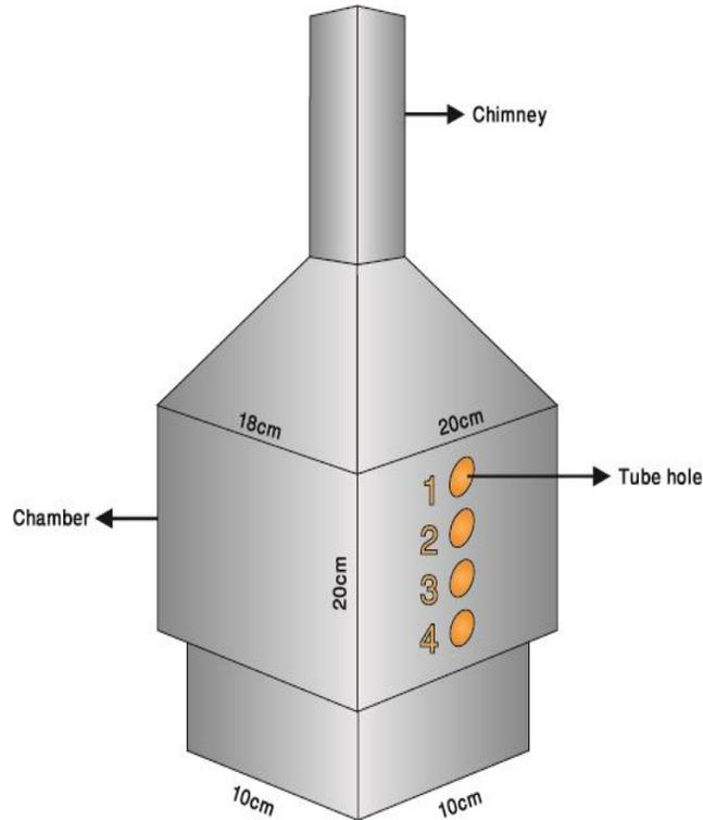
Figure. 1. Schematic diagram of the Chimney Type Fire Tube Heat exchanger with dimensions.
