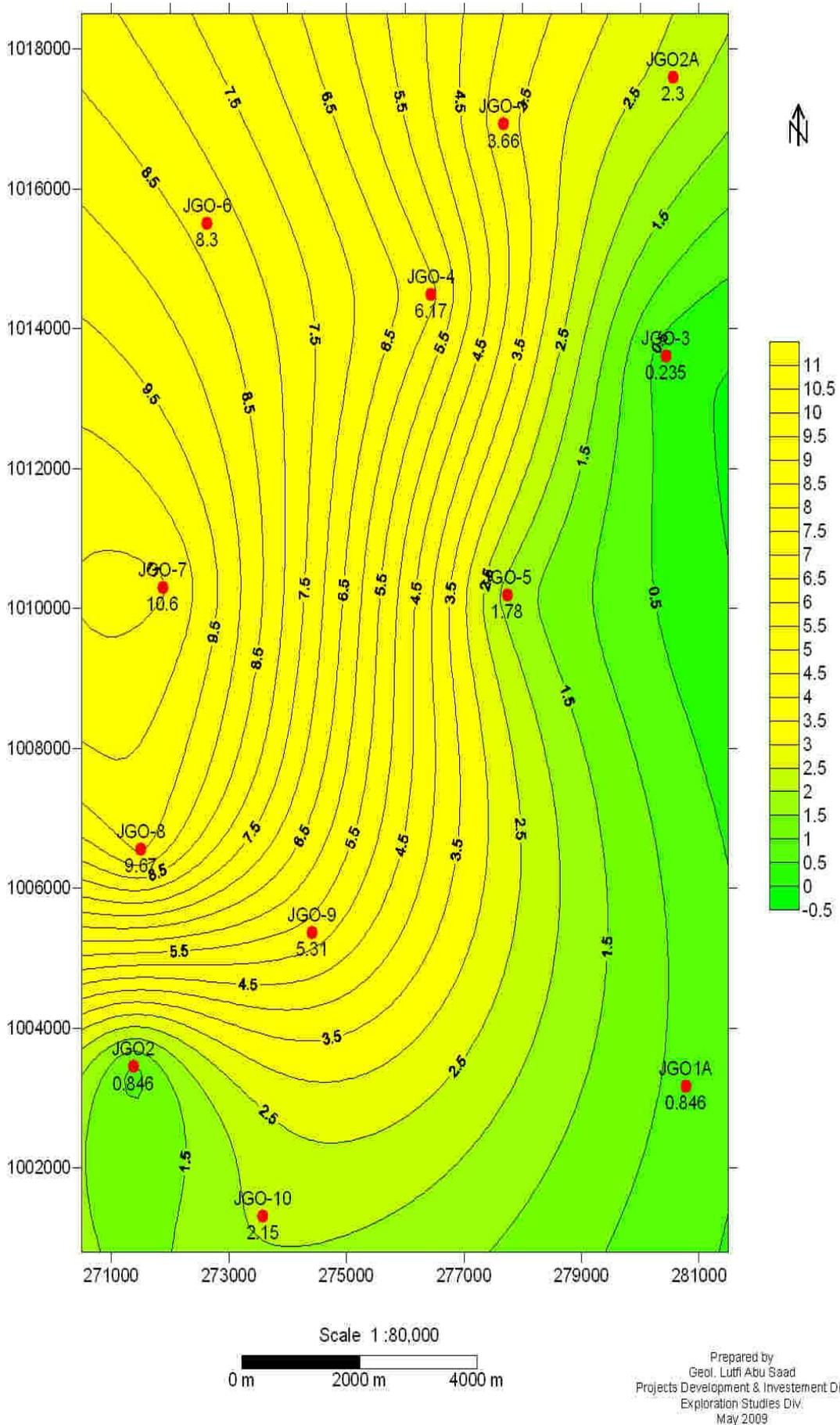
Fig. 5: Isoline map of stripping ratio.
