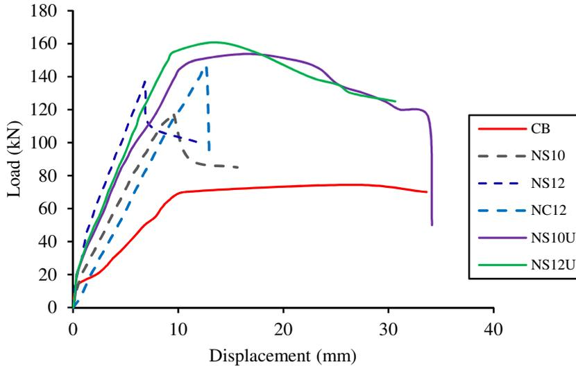
Fig. 3: Load vs. displacement at mid-span for all beams.
