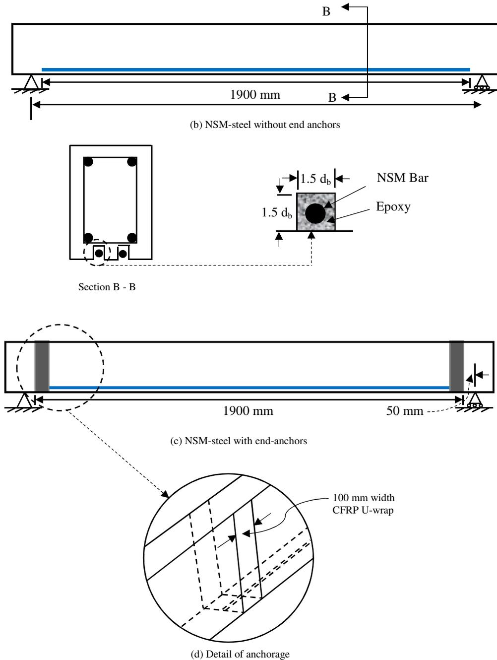
Fig. 1: Beam specimens details
