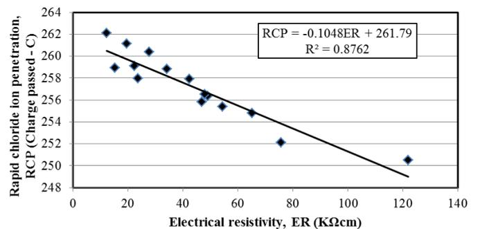
Figure 9. Correlation between electrical resistivity and rapid chloride ion penetration
