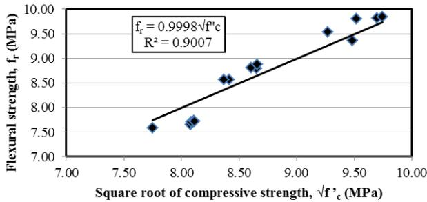
Figure 2. Correlation between compressive strength and flexural strength
