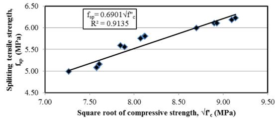
Figure 1. Correlation between compressive strength and tensile strength
