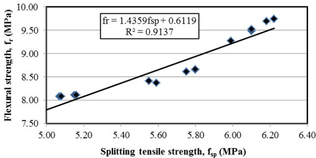
Figure 3. Correlation between tensile strength and flexural strength
