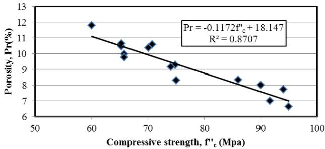
Figure 6. Correlation between compressive strength and porosity
