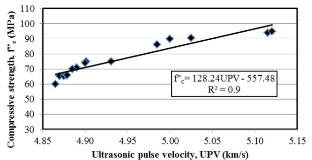
Figure 5. Correlation between compressive strength and Ultrasonic pulse velocity
