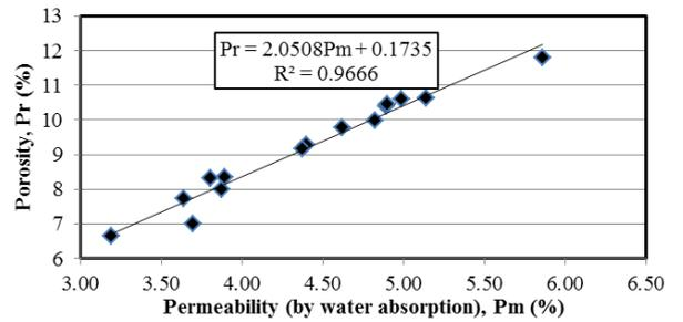
Figure 8. Correlation between porosity and permeability (by water absorption)
