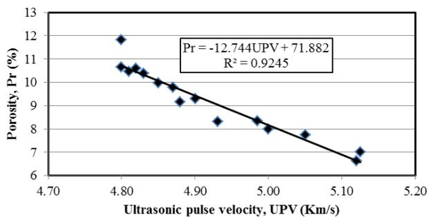
Figure 7. Correlation between Ultrasonic pulse velocity and porosity
