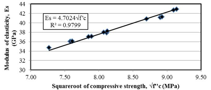
Figure 4. Correlation between compressive strength and modulus of elasticity
