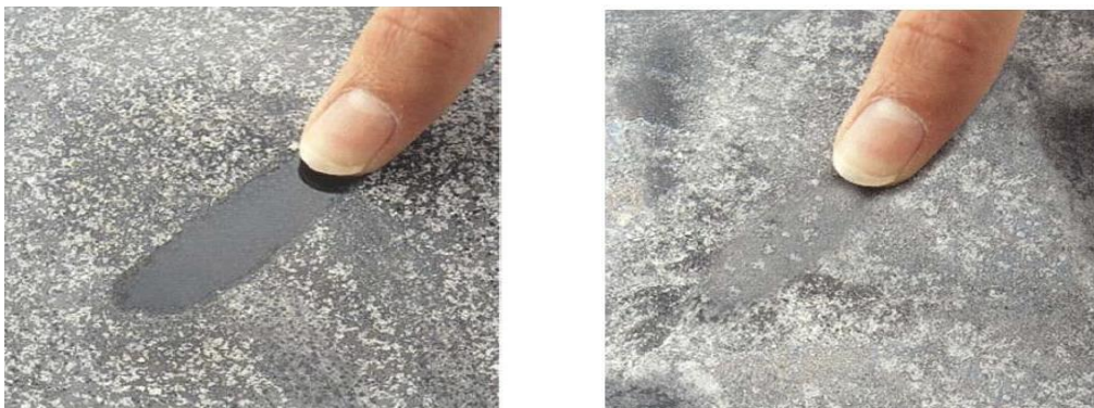
Fig 11: A comparison of ceramic surfaces – left without ETC coating, right with ETC coating. Flexible ETC ceramic wall coverings, similar to wallpapers, can withstand direct exposure to water, such as that in a shower cubicle thanks to their highly Water-repellent surface. Source: www.forbes.com
