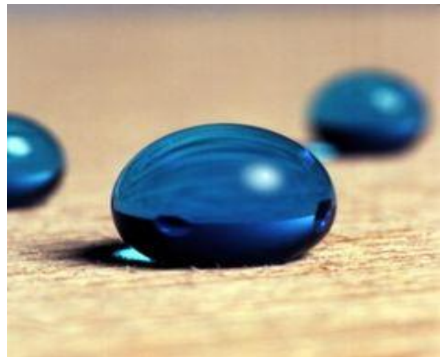
Fig 5: Wood can be given an extremely water-repellent self-cleaning surface.
