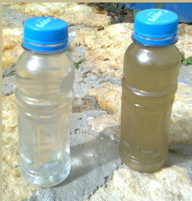
Figure -13 photo showing the wastewater before (right) and after (left) treatment process.
