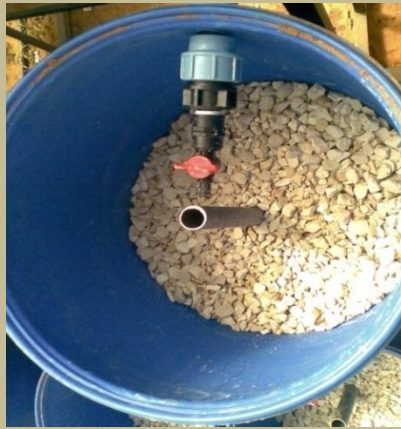
Figure (4) constructed wetland with total height for media equal to 50 cm
