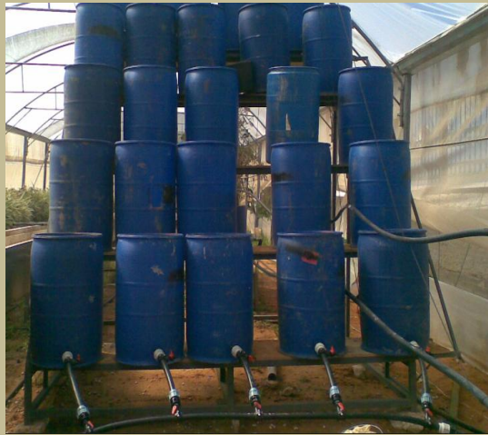
Figure (2) Constructed wetland system with vertical flow (4-stages) for treatment.
