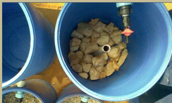
Figure (3) The first layer in the constructed wetland is gravel for a 13cm-height.
