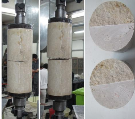
Fig. 3 Fracture and growth of failure in DT specimen
