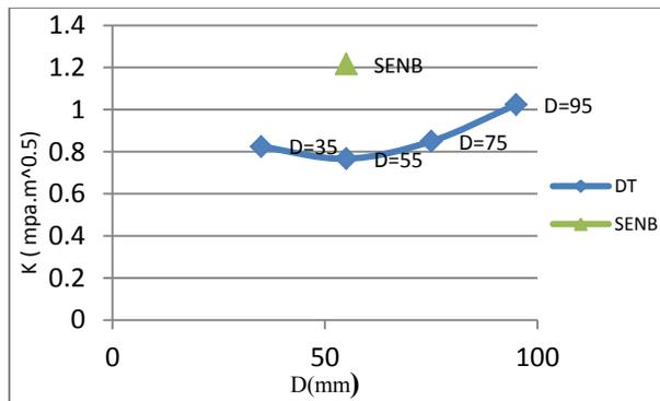
Fig. 6  $K_{IC}$  results obtained from two DT and SENB methods.
