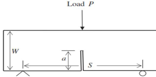
Fig. 2 Geometry and loading of the cubic specimen for SENB test [11]
