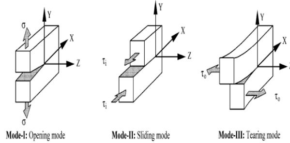
Fig. 1 Basic fracture modes
