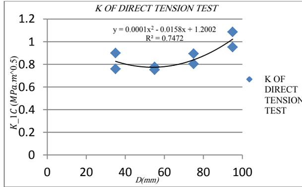
Fig. 5 variation of fracture toughness by variation of diameter in DT specimen.
