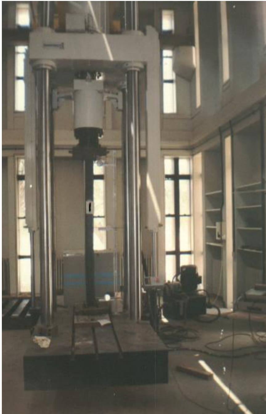
Figure 2 : Load Application on Column Specimen.
