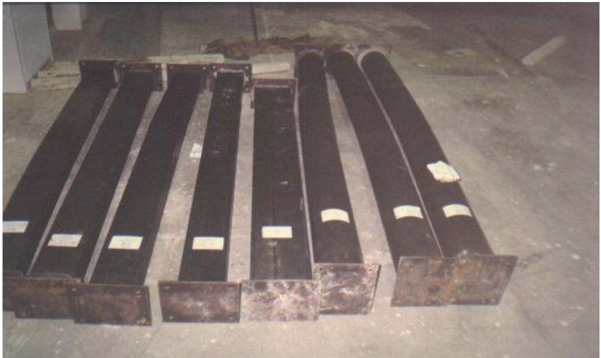
Figure 5 : Mode of failure for some of the tested columns .
