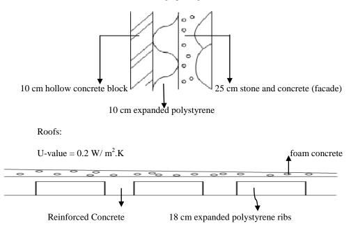
For the solar heating of the house with the above cross sections, 12 solar collectors and 4 fan coils are needed.
