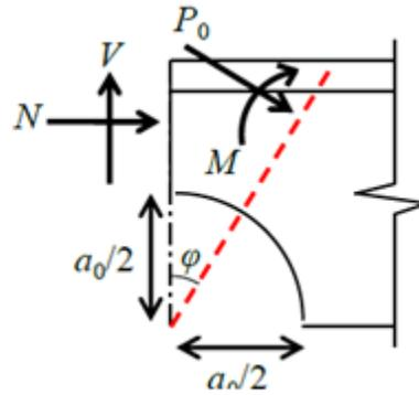
Figure 5. Vierendeel Bending in Critical Section
