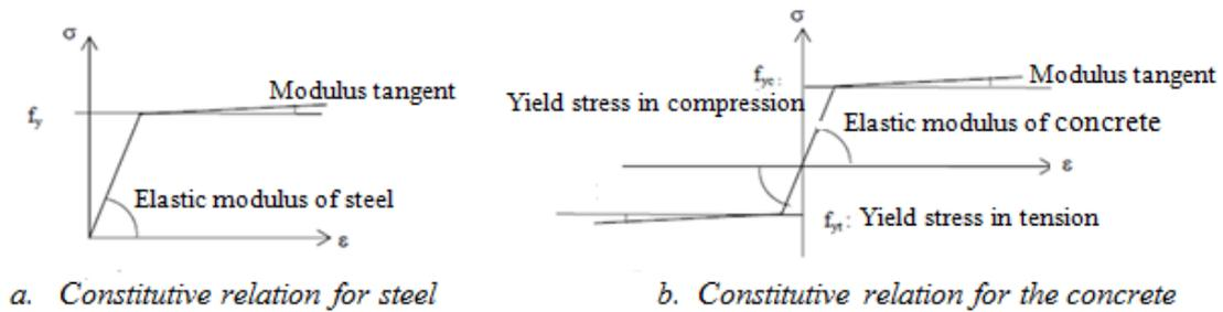
Figure 4. Stress-Strain Curves
