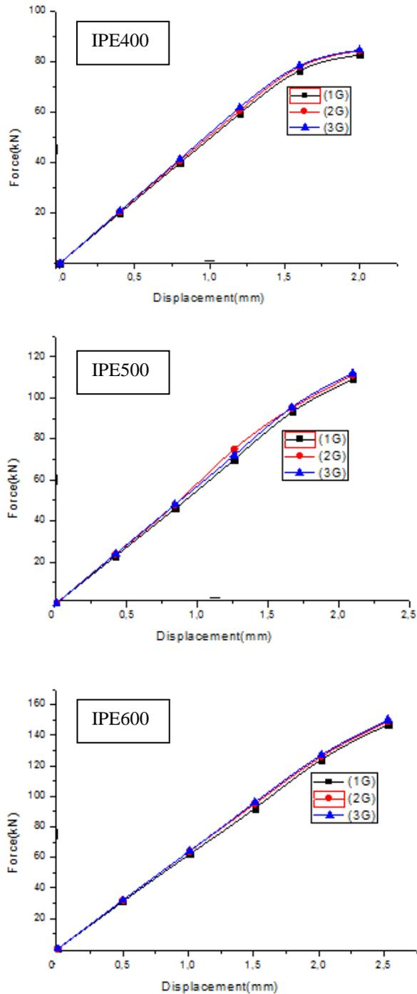
Figure 9. Behavior Force-Displacement at the Opening (n°4).
