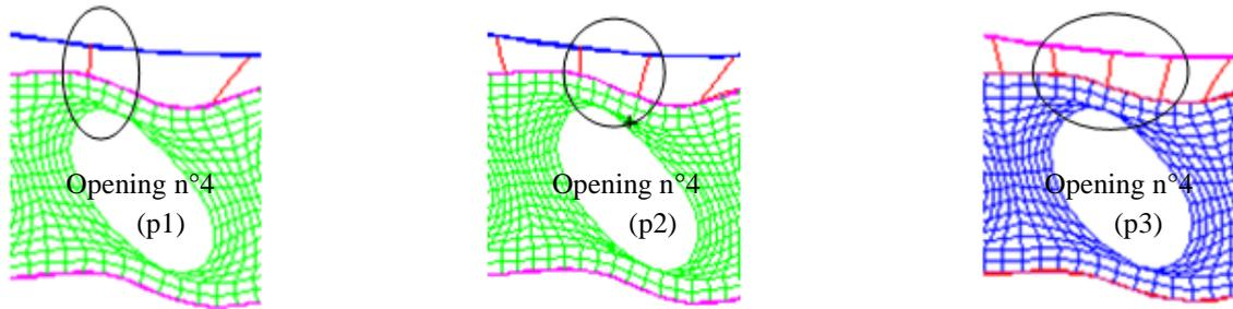
Figure 8. Plastic Hinge in the Upper Member of the Beams (p1, p2, p3)
