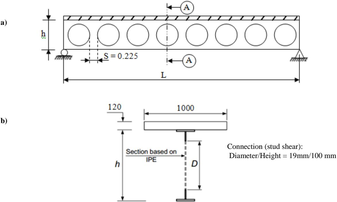
Figure 2. Composite Cellular Beam: a) Static Scheme, b) Cross-Section (A-A)
