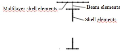
Figure 3. Finite Element Modeling
