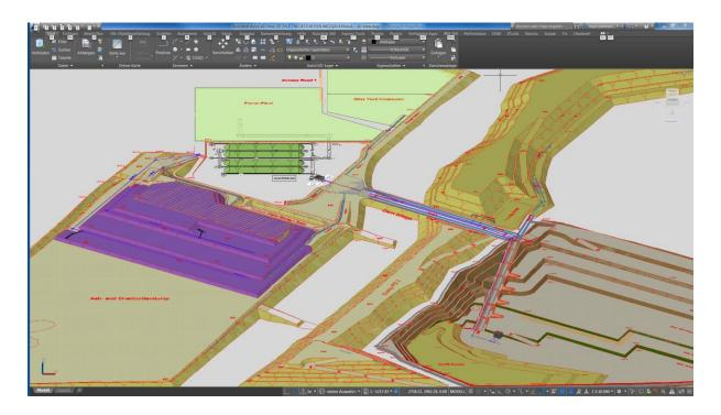
One of the key topic for inhomogeneous deposits is the optimised blending calculation of different loading points to ensure the quality supply and economic efficiency of the short term mining operation which can be solved by a derived mine block model from the geological block model.
