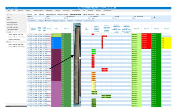
The type of the modelling methods becomes important and depends on the nature of the deposit. For sedimentary deposits like limestone and oil shale a layer-bound/stratigraphic block modelling is suitable. Contrary to conventional block models the stratigraphic block model considers arbitrary formed layer boundaries and thus simulates the real deposit conditions which have been developed during sedimentation of the material bearing seams.
