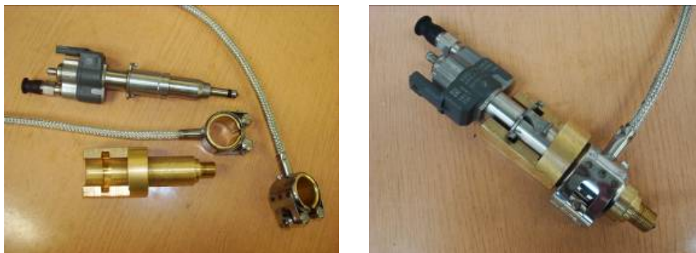
Fig. 1. An injector fitted with a fuel heating system
