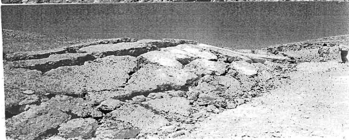
Figure 8. July 10, 1995 landslide at WESTP project, (a) the 2 to 8m deep scarp with the sliding surface along the moderately dipping stratum of plastic clayey marl underlying the jointed weathered limestone, (b) the heave at the toe of the rotational slide in the plastic clayey marl.
