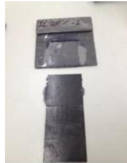
CFRP Laminate debonding of 20%IL
