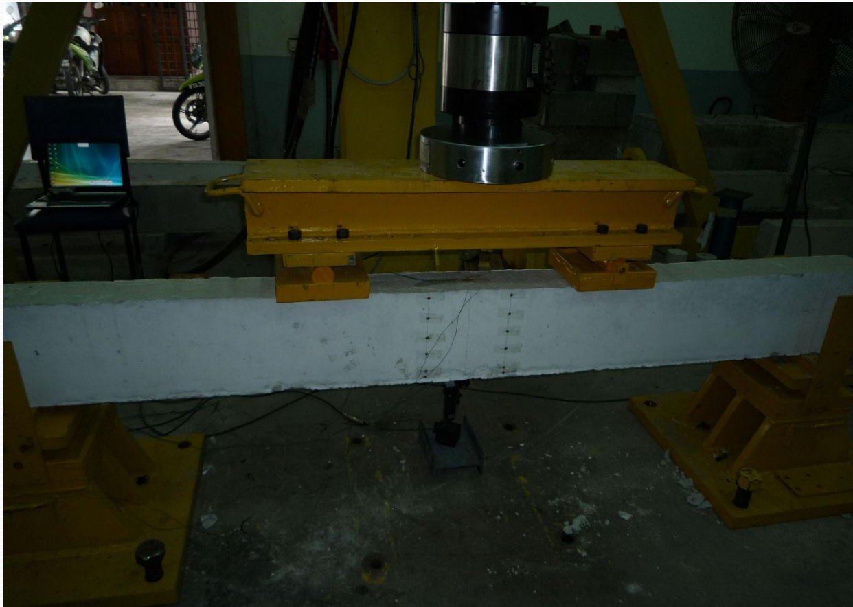
Fig. Instrumentation and loading set-up.
