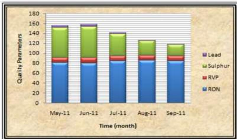
Fig.5. Changes in Iraqi gasoline blends' specifications
