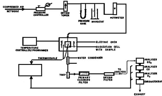
Figure 4: cell oxidation Apparatus
