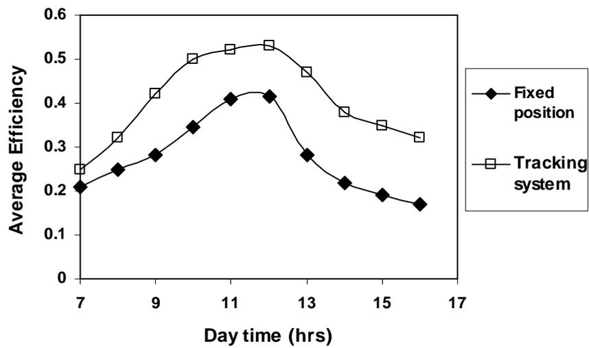
Figure 6 Average efficiency for cookers at fixed and on tracking systems for the three working days
