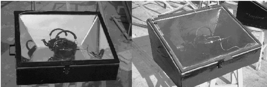
**Figure 1 Tested solar cookers: a) Black painted box type cooker, and
