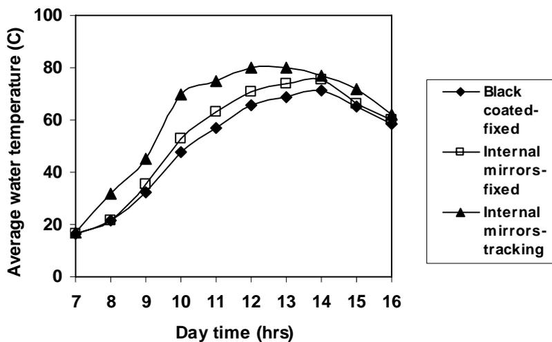
Figure 4 Average water temperature for the three proposed systems at the three working days.
